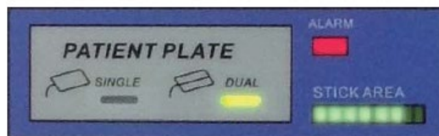
Neutral electrode recognition & contact area monitoring and display
