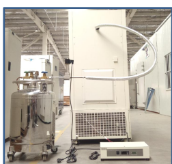
LN 2 /CO 2 backup system
